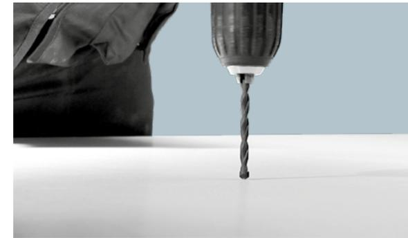
8 | As far as manual drilling is concerned, use tungsten bits with a diameter up to 10 mm, fitted to electric drills or battery-operated screwdrivers.
