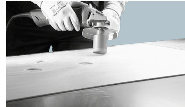
9/10 | As an alternative, one can use holesaws fitted to angle grinders, electrical drills or battery-operated screwdrivers.
