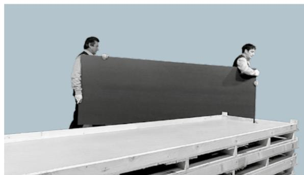
3 | When the slab is upright, hold it from its top edge and shift it keeping it straight and upright. This operation should be performed with the aid of a second person.
