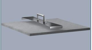
3/4 The handle is equipped with two 4 mm thick side hooks, so that it can be inserted between the joints and easily lift the tiles that are already laid. Available in different sizes, the practical galvanized steel handle facilitates the installation and maintenance of elevated floors.
