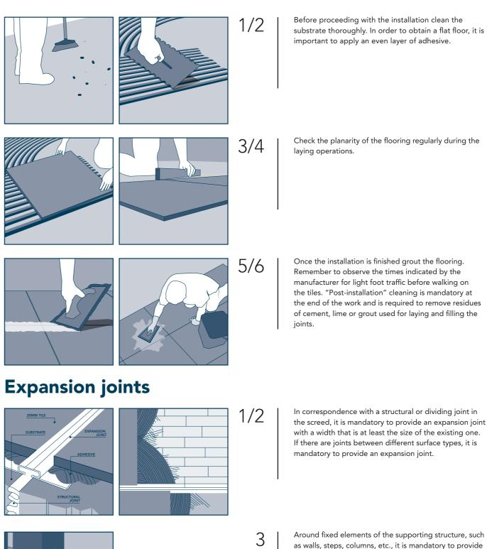
peripheral joints with a width of between 4 and 12 mm.
